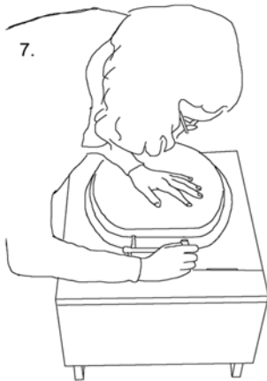
7. Mark holes for toilet seat attachment.
